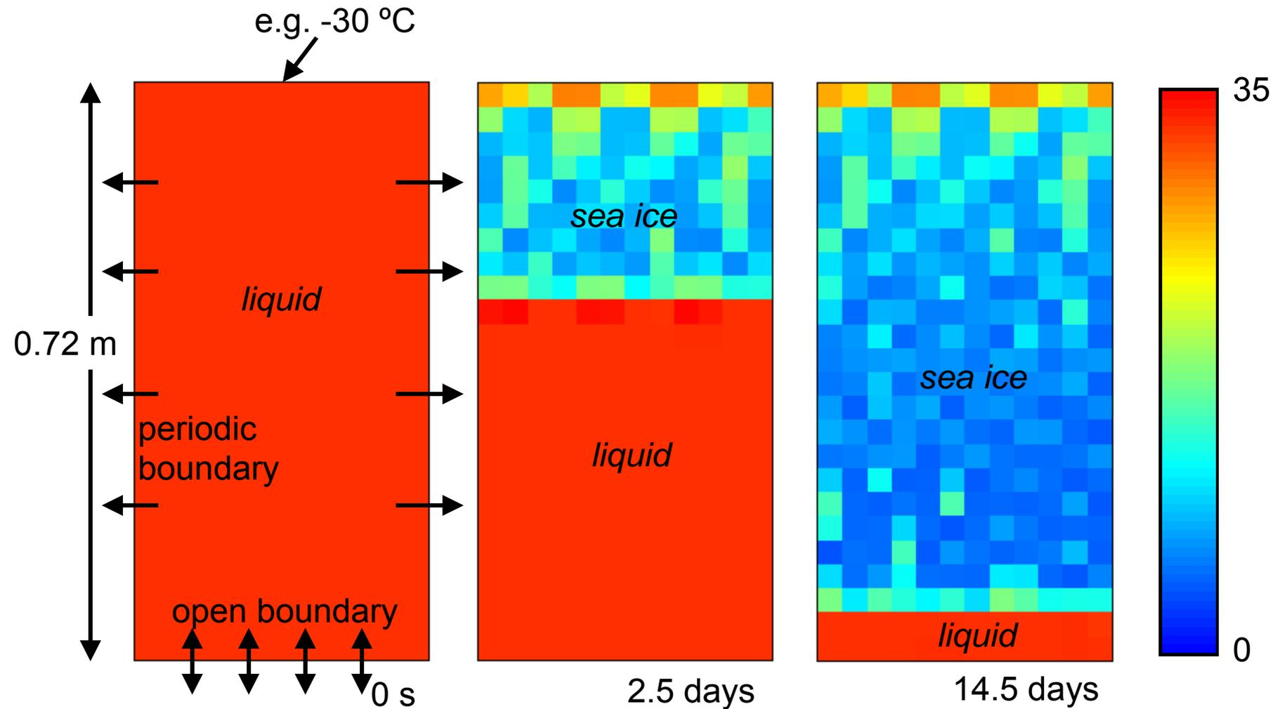
Temperature of brine entering domain: 10 mK above freezing point
