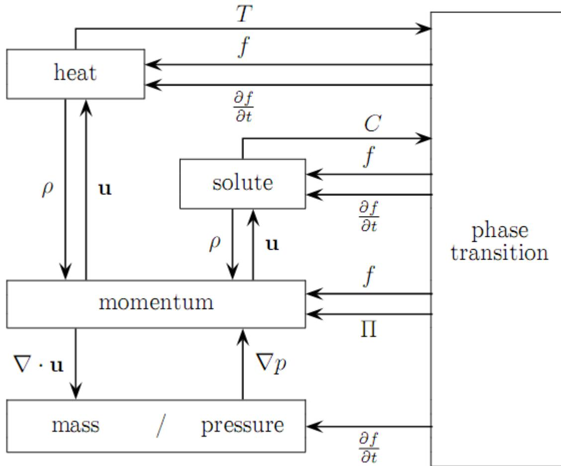
Solved on staggered, rectangular grid w/ multigrid solver
